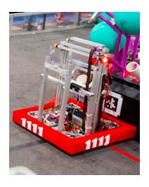
For the 2025 FRC game, Reefescape, the Power Hawks built our robot Osprey. This bot operates with a 3-stage elevator to place a piece of coral (PVC pipe) on all 4 levels of the reef (metal bar structure). Together, we create an alliance with 2 other robots to compete against the other side for who can get the most points through scoring game pieces and completing specific challenges like "coopertition<sub>®</sub>" and maneuvering to a set position during endgame.
